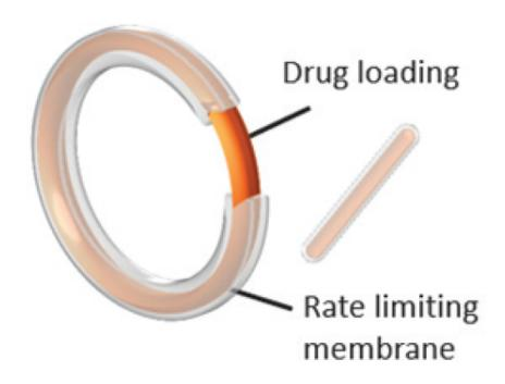
VitalDose EVA Implant with Core layer (reservoir) and a Membrane layer (raye limiting membrane)
